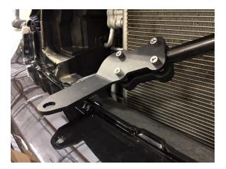
7. The positioning of the brackets is important, so take some time now to get the brackets mounted level, and centered on the car. The inside edges of the light tab should be 21" apart. This should result in the tabs resting about an inch off of the top surface of the bumper.
