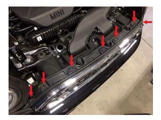
5. With the screws out, gently pull the grill forward slightly to reveal several tabs that secure the bottom to the bumper. To disengage the clips, push down on the tab while wiggling the grill outward.
