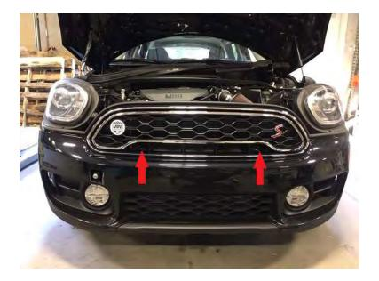
4. We will need to remove the grill. Start by removing the 7 T30 Torx screws across the top of the grill.
