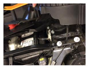
3. Now we can access the battery box lid. It is secured by 2 8mm screws. Remove the lid and disconnect the negative battery terminal by loosening the 10mm bolt on the clamp. Once you've disconnected the cable, it's a good idea to secure it to the support bar to make sure it doesn't come into contact with the terminal while you're working.
