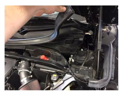
2. Once the seal is removed we can also remove the "s" shaped plastic piece, this will help with wire routing down the line. Use the trim panel tool to pop the clip, and then the whole thing will come off.
