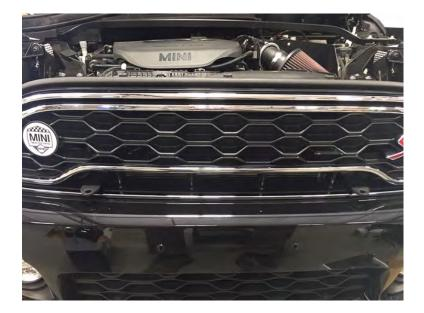
9. Set the grill back into place. Use the palm of your hand a gently bump the grill along the bottom edge listening for the telltale sound of the tab clips clicking back into place. Now you can reinstall the 7 T30 Torx screws along the top and side of the grill.
