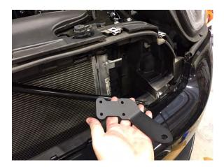
6. Grab a bracket and insert one of the 1/4-20 x 1.25" cap screws through each of the four holes. Hold the bracket and dogbone in place on the cross bar, and finger tighten the screws into the dogbone.
